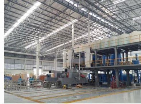
Paste mixing and plate coating
