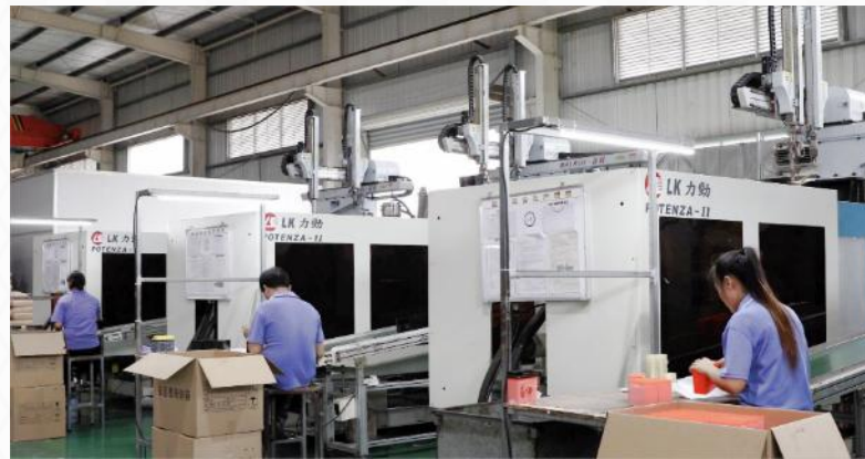
Battery Case injection molding
